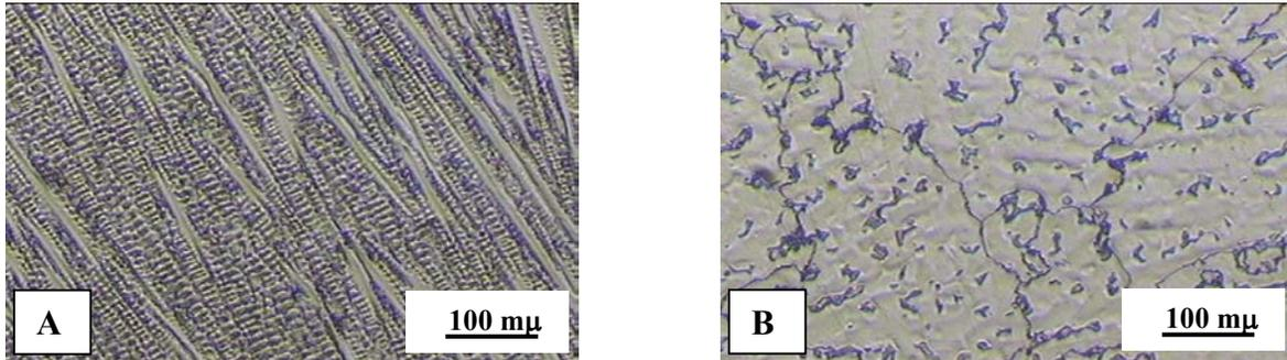
Figure 1. Microstructure of CoCrMo alloys: (A) Vitallium, (B) VeraPDI
