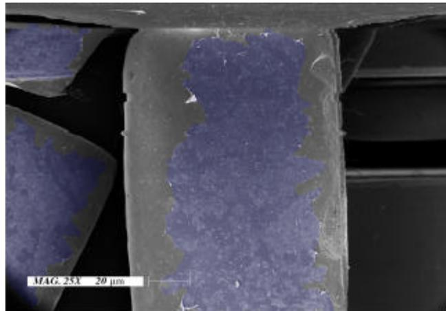
Figure 10. SEM image of duceragold specimen. The pseudo-coloured area is covered by cells.
