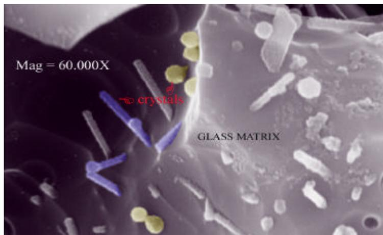
Figure 1. Micrograph of feldspatic ceramic. The crystals and the glass phases are visible.
