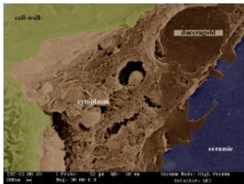
Figure 14. SEM image of duceragold samples with A-431 cell after cell body fracture.
