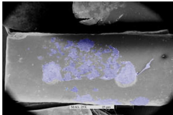
Figure 10. SEM image of duceram specimen. The pseudo-coloured area is covered by cells.
