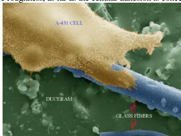
Figure 15. SEM image of duceram samples. In blue two glass fibres “attached” to the ceramic surface that belongs to the firing support. The only one cells present on this area is strongly attached to them.
