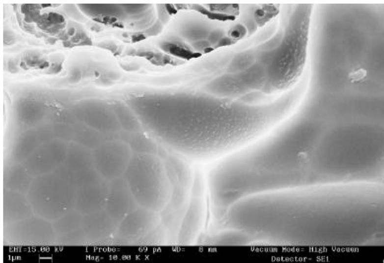
Figure 2. Micrograph of glass ceramic. The generous glass phase is visible.
